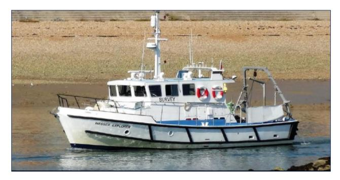
Survey sensors will be towed up to 100m from the stern of the vessel. Therefore, all mariners are requested to pass well clear of the vessel. The Wessex will maintain a listening watch on VHF channel 12 and should be contacted to arrange safe passing where necessary.
