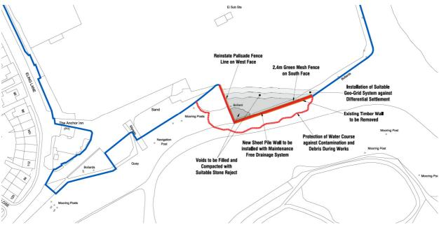
These emergency works comprise the installation of a new sheet pile wall behind the existing structure prior to removing the damaged and eroded timber sections. The programme is scheduled to commence on Monday 22<sup>nd</sup> August 2022 for a planned duration of 10 weeks.
