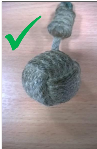
Figure 1 - MCA Notice, Dangerously Weighted Heaving Lines
